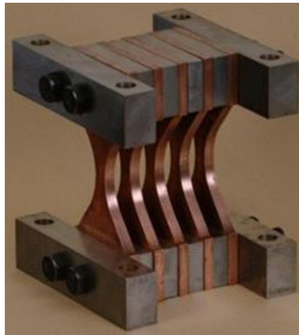
Figure 8.5: Example of an ADAS hysteretic (or yielding) energy dissipator. Seismic energy is dissipated through the plastic deformation of the curved metal plates.
